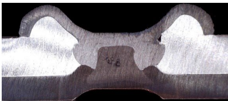
Figure 1 – Cross section of 3.8 mm Aluminum Die Casting joined to 2.0 mm Press Hardened Steel using RSR from 2024
