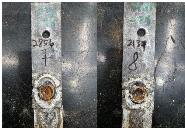
Figure 2 – Untreated RSR Samples that were salt spray tested and then pulled in tensile shear, to be presented at SMWC
