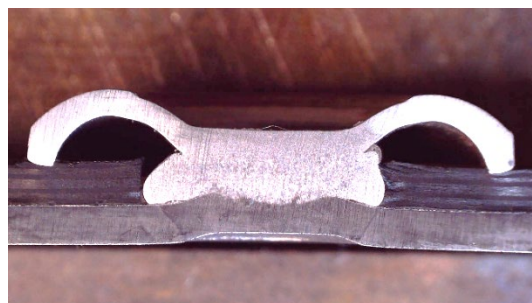
Figure 1 – Cross section of 1.6 mm CFRP jointed to 1.5mm Usibor1500 using RSR
