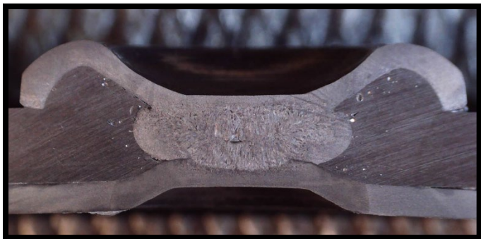
Figure 2 – RSR Cross Section: 3.0 mm ADC to 1.2 mm 980 MPa GA Steel
