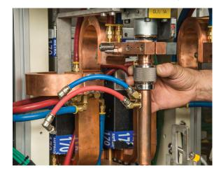
New Tooling Platen with Automatic "Locate & Lock"
