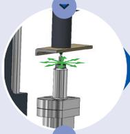
Actuator is extended, LPT and VeriFast™ IA confirm a fastener is present and in the correct orientation to be clinched.
