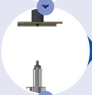
Clinch pin is extended into the hole in the workpiece. The profile of the clinch pin allows the floating C-Frame to align to the workpiece ensuring the fastener and hole in workpiece are concentric.
