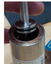
**14** Ensure that the Weld Pin moves freely up and down inside the Weld Body (with no constraint from the LVDT Cable Assembly), then attach and tighten the Weld Head.
