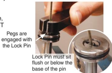
**12** Apply Magnalube-G grease to lubricate the O-Ring on the new Weld Pin.
