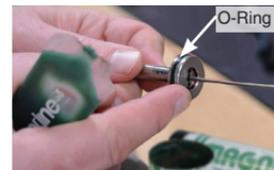
**13** Gently insert and fully slide the LVDT Cable Assembly through the hole in the bottom center of the Weld Body, until the Weld Pin properly sits inside the Weld Body.
