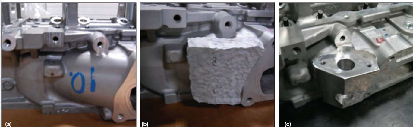
Fig. 3 — Freeform feature added to a prototype machine component by cold spraying. (a) Prior to spraying, (b) as sprayed, (c) finished.
